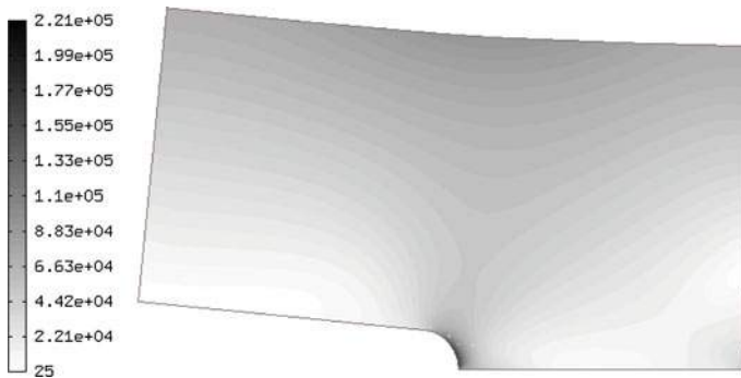
Fig. 15 Output of the linear elasticity example—von Mises stress
